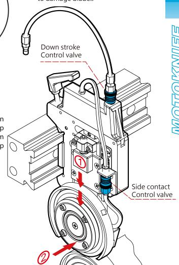
Individual valve control More convenient for down stroke and side contact individual valve control, it can be operation under automatic action or separate when
